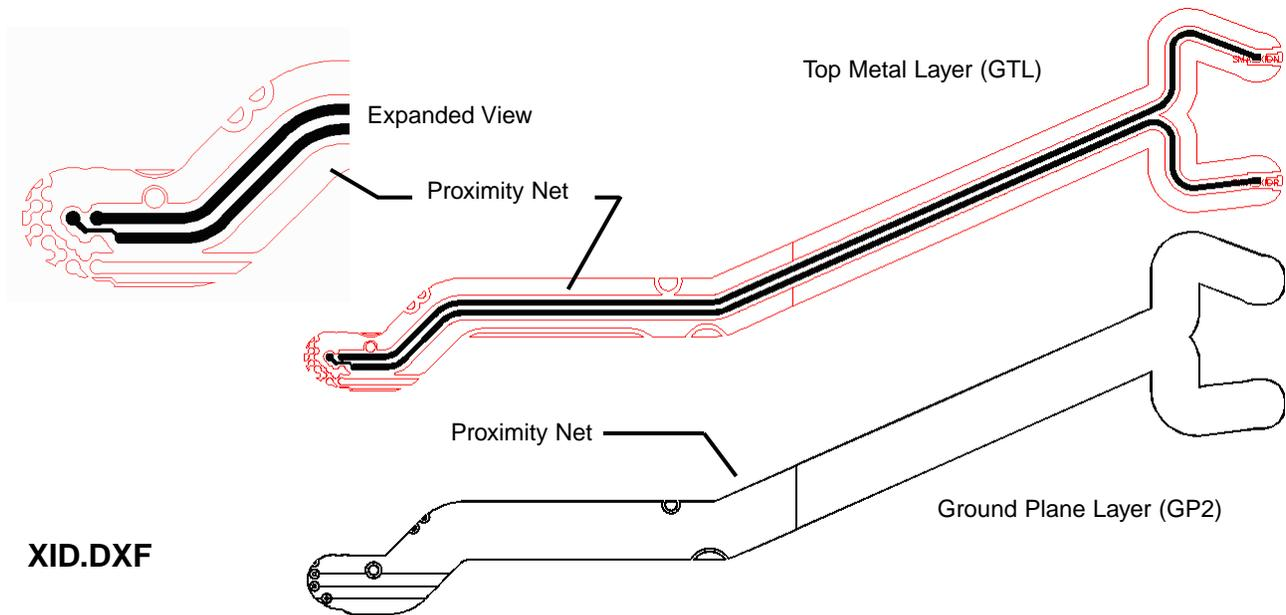
We requested two nets: XIDP and XIDN (the positive and negative halves of a differential pair) and also requested a proximity net that extends 0.070 inch out past the nets.
