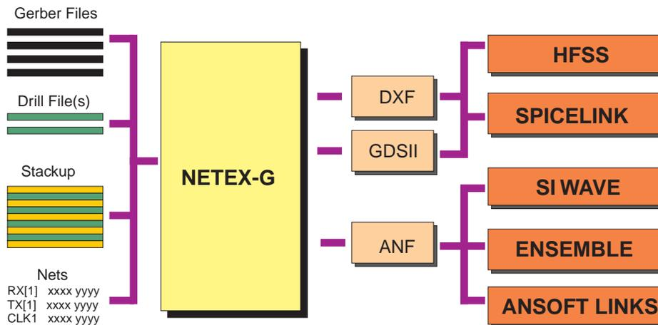
Gerber Data provides the conductor geometry
