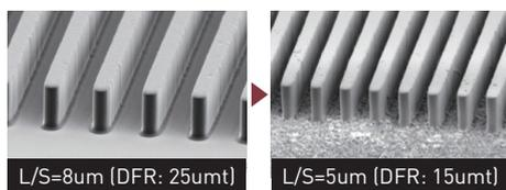
repeated unique improvements to the patterning engine optical system. Research and development is continuing for a change from the current  $L/S=8\mu\text{m}$  to  $L/S=5\mu\text{m}$ . Furthermore, a scan speed 1.4 times that of conventional models has been achieved, resulting in substantial improvements in productivity while also enabling a pattern positioning precision of  $|AVE|+3\sigma<7\mu\text{m}$ .
