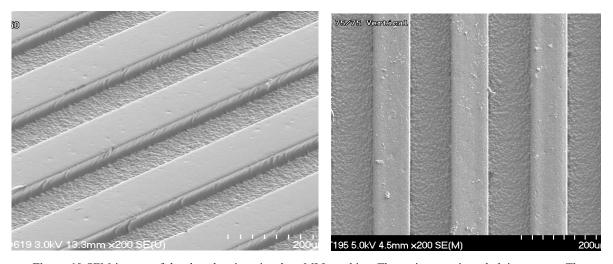
**Figure 10** SEM images of developed resist printed on MLI machine. The grainy area is underlying copper. The features are 75um lines and spaces.
