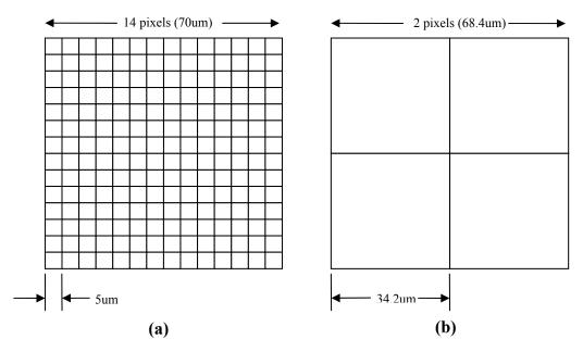
**Figure 9** Comparison of pixel sizes in a binary "dot matrix" style scheme and gray level scheme that both provide similar feature placement resolution. (a) Binary pixels for feature placement of +/-2.5um. (b) MLI gray level pixels for feature placement of better than +/-2.5um. There are ~49 binary pixels for every gray level pixel.
