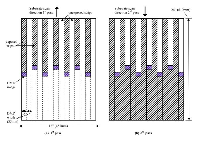
**Figure 4** Scanned exposure of a typical PCB panel for a 7 channel system. Projected DMD images are staggered by the width of one image. Two interlaced passes are needed to cover the area. (a) First pass (b) Second pass
