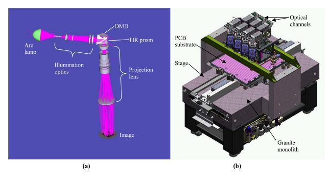
**Figure 3 (a)** Optical layout for a single channel. **(b)** Channels as integrated into a 7-channel machine. Channels are shown mounted above the precision stage that moves the substrate.
