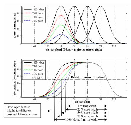
**Figure 8 Simulation of gray level edge control.** Upper graph shows dose profiles for 4 blurred mirror images on 30um pitch. The leftmost dose profile is shown for 4 different dose levels. The lower graph shows the corresponding effect on left edge placement and developed feature width versus left mirror dose.
