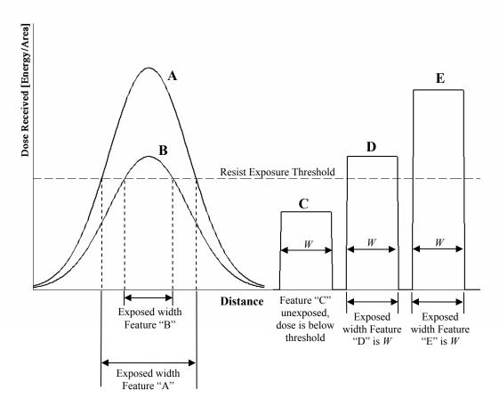
**Figure 7 Gray Level Imaging.** Dose profiles "A" and "B" are examples of Gaussian profiles that might be produced by a "blurred" intensity distribution incident on a photoresist. For these profiles the exposed feature width changes with dose once the resist threshold is crossed. For sharply resolved or "tophat" profiles "C", "D", and "E", the exposed feature width does not change with dose. Hence, a somewhat blurred dose profile is crucial to gray level width control.
