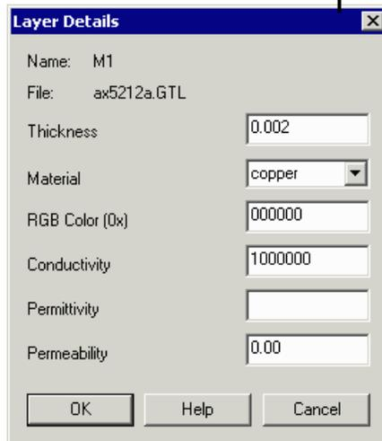
Layer Details: every layer can be assigned a thickness, material and electrical properties. These are not mandatory for NETEX-G but other programs may want to read the values for electrical analysis.
