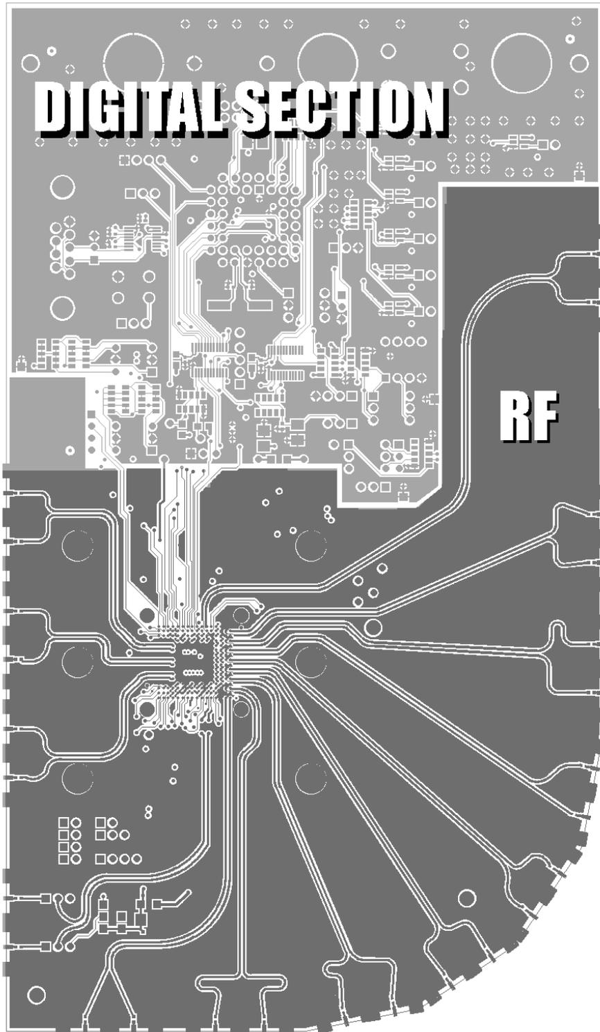
Our goal is to analyze all of the controlled impedance differential pairs that connect the outside world to the IC.
